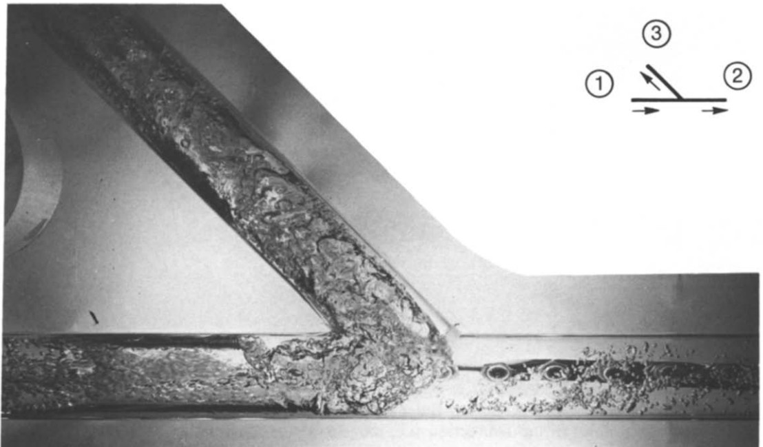
Figure 5. Phase separation—dividing Y-junction (135°, top view). w_1 = 1.579 (kg/s), x_1 = 0.2001 (%), w_3/w_1 = 0.5172 , x_3/w_1 = 1.810 , p_1 = 0.1359 (MPa).
