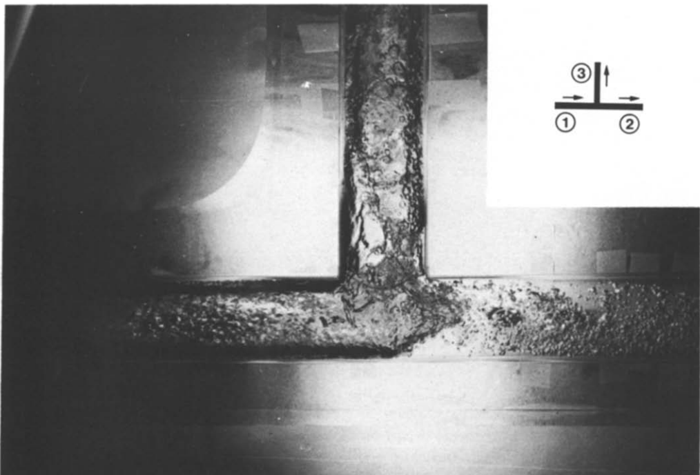
Figure 3. Phase separation—dividing T-junction (top view). w_1 = 2.284 (kg/s), x_1 = 0.2106 (%), w_3/w_1 = 0.3108 , x_3/x_1 = 2.608 , p_1 = 0.1484 (MPa).
